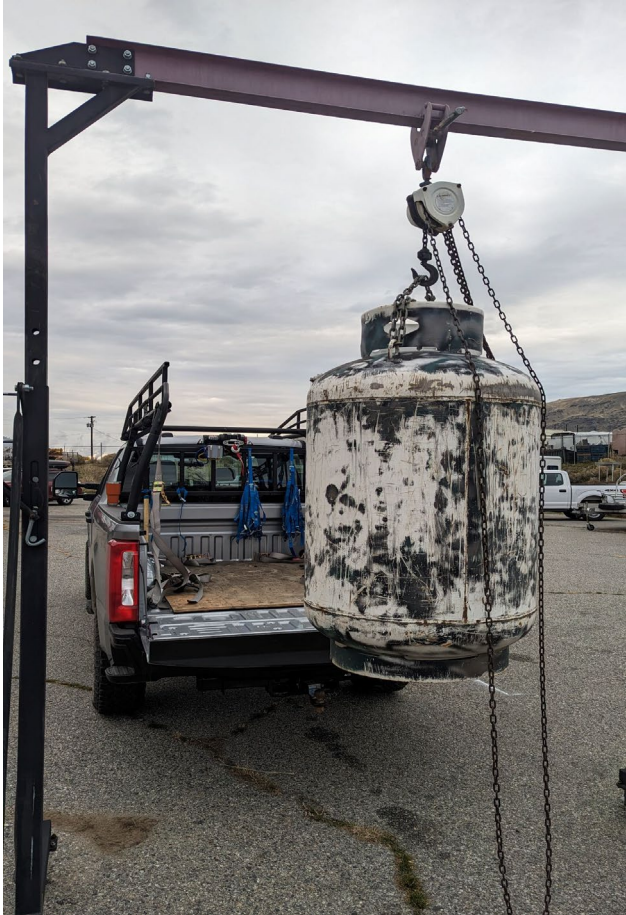
Chain hoist for loading/unloading @office
